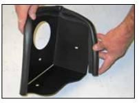
8. Install the provided edge trim onto the heat shield as shown.
