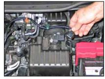
2. Disconnect the mass air sensor electrical connection and unhook the wiring harness from the factory air box.
