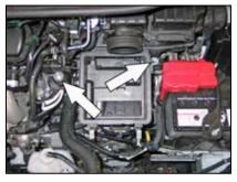
4. Remove the two air box mounting bolts shown.
