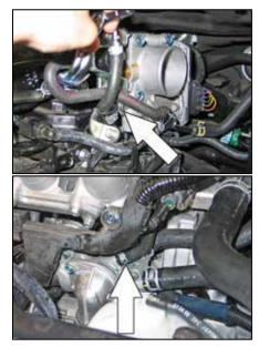
14. Be sure the engine is cool and the cooling system is not under pressure. Loosen the hose clamps and remove the coolant bypass hose from the throttle body and thermostat housing. Be sure to capture any lost coolant in an appropriate container.
