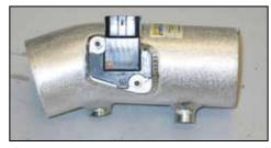
18. Install the mass air sensor into the  $K\&N^{\otimes}$  intake tube and secure with the provided hardware.
