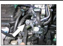
13. Release the spring clamp which secures the crank case vent hose to the valve cover and disconnect the vent hose from the valve cover.
