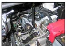
3. Release the four upper air box retaining clips and then remove the upper air box from the vehicle.
